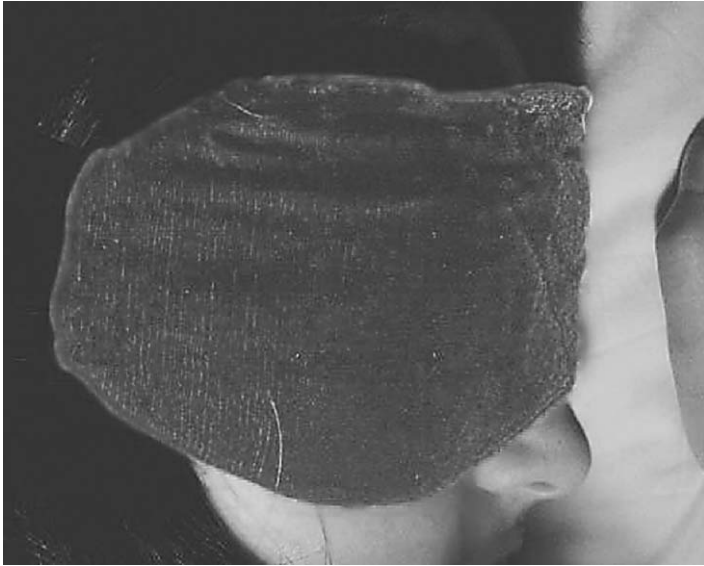
Figure 13.11 The Aura prototype sleeping mask with integrated electro-oculargram.
