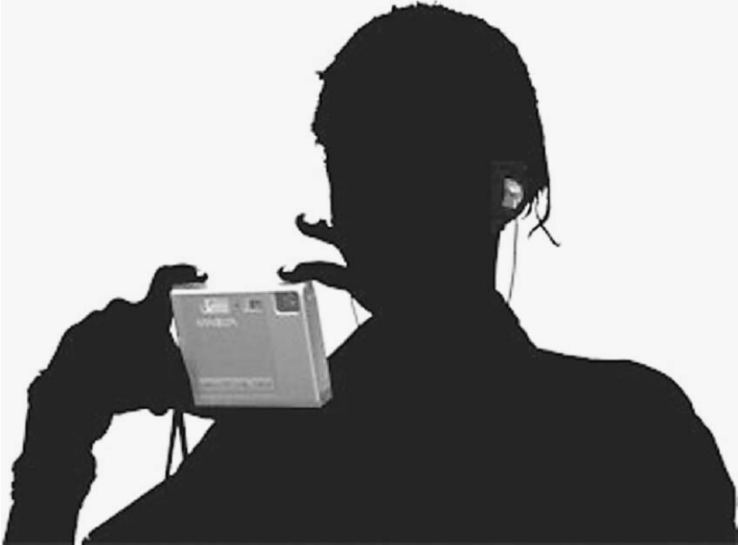
Figure 13.30 Depiction of the RAW audiovisual recording tool, consisting of a digital still camera and ear-microphones for binaural audio recording.
