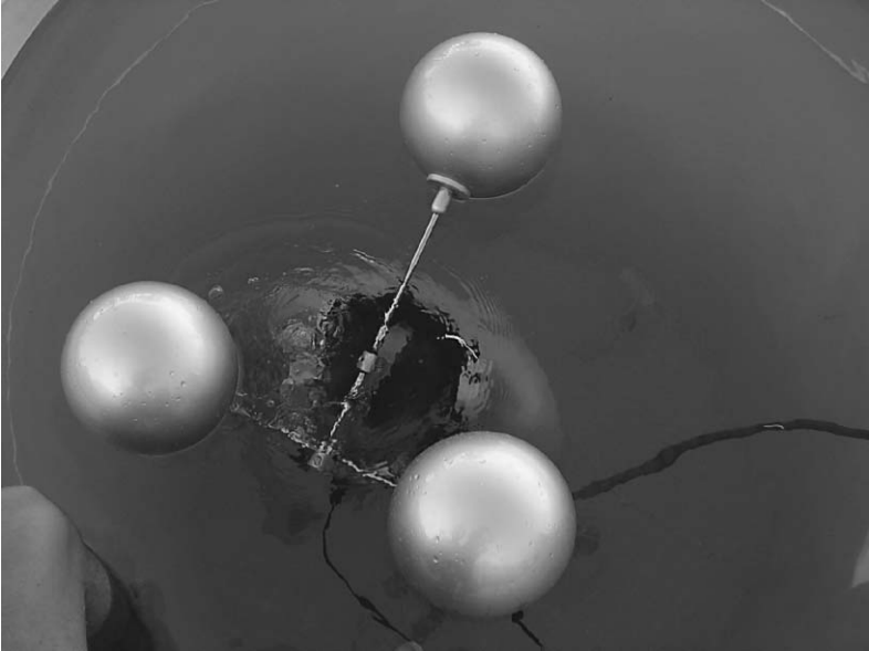
Figure 13.18 Iso-phone mask in use completely under water.
